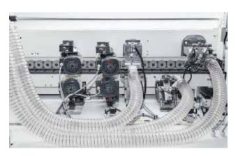
Double polishing device: meets the coating requirements of two different colors and improves the surface appearance quality. standard 1 pic polishing device.
