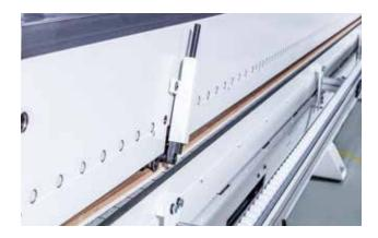
The steel upper pressure beam and V-belt are tightly pressed to ensure smooth delivery of the workpiece
