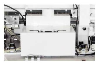
Joint trimming unit: Perfect cut and long service life due to diamond tipped tools for optimum edge joint quality.
