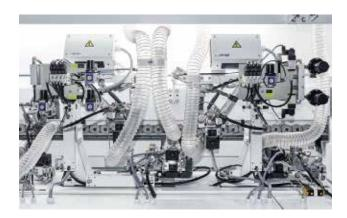
**Profile trimming unit:** For profile trimming of thick PVC edges. Workpiece thickness up to 60 mm. Standard pneumatic on/off. For easy operating. Max. feed speed 25 m/min.
